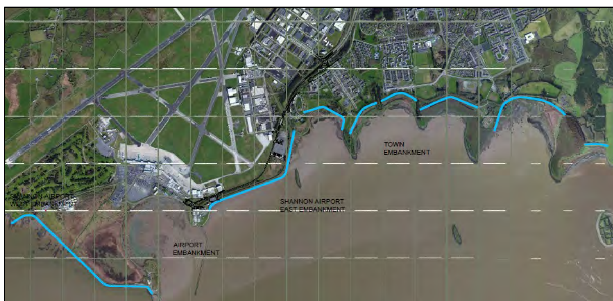
Plate 5-3: Location of Flood Protection Embankments
