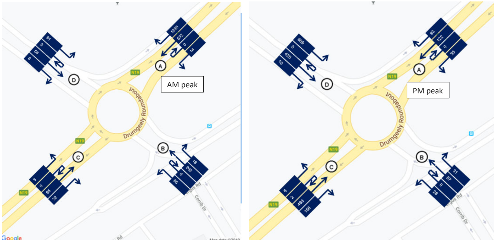
Figure 3-4: Peak flows at Drumgeely roundabout
